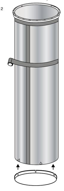
Attach the diffuser to the bottom extension tube, then slide the assembled system down through the roof flashing.
