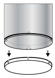
Attach the diffuser to the bottom extension tube, then slide the assembled system down through the roof flashing.
