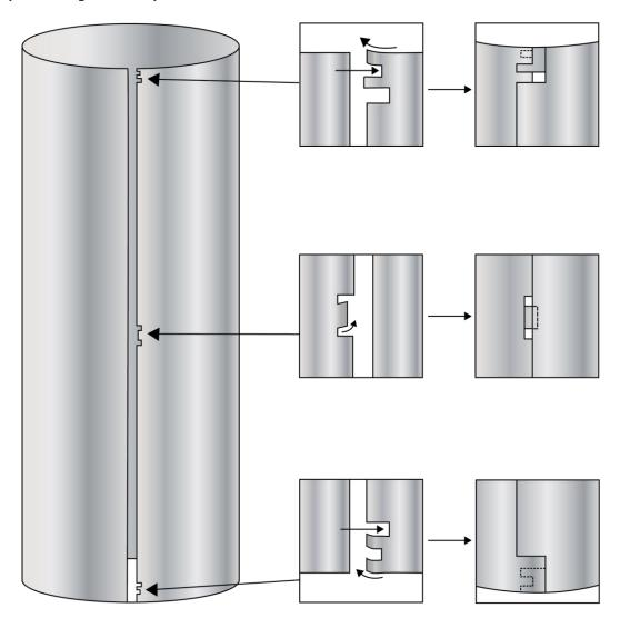
Tape the entire length of the tube seam with aluminium tape on the outside of the tube. Remove the protective film from the extension tube
